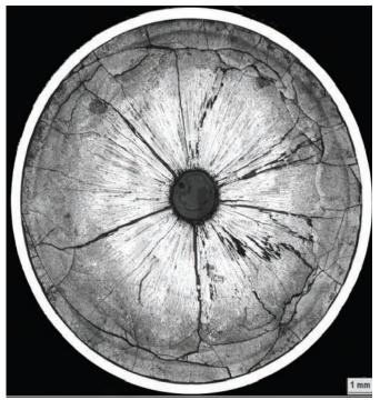
Micrograph of an irradiated, failed fuel pellet showing the restructuring in fuel.
