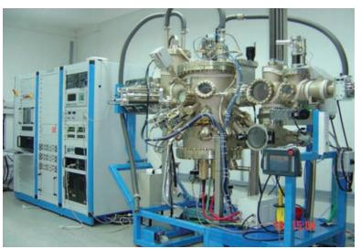
MBE facility for growth of silicon-germanium based quantum well structures.
